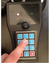
7. After entering the 5-digit code, press the '#' key. The red indicator will light steady again.
