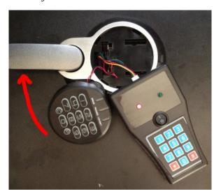
6. Wait for the red indicator to light up. Once it has lit up, enter the 5-digit code that you want to program to the safe. Note that upon entering the first digit, the red indicator will turn off, and blink for the succeeding digits that are pressed.
