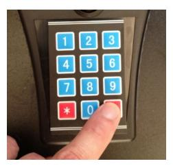
8. Wait until the **green** indicator lights up, then pull the lever all the way down to open the safe. Usually, the clicking of the energized solenoid can be heard as the indicator LED turns green.
