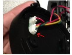
4. Plug the 4-wire connector to the socket located at the top portion of the Dumb Safe Opener tool.
